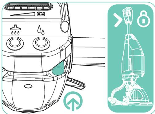
Use the button located at the rear for quick locking while in cleaning mode.
