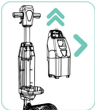
Remove the tank from the machine, using the inset handle.
