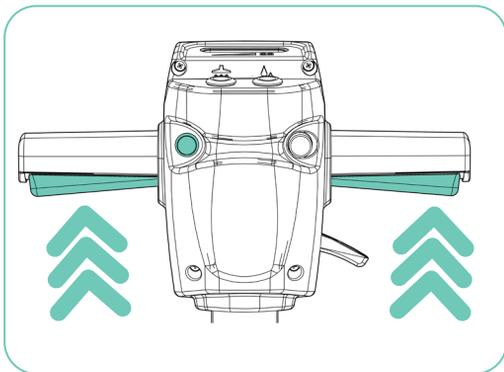
To start the machine pull both handle levers in and press the start button.
