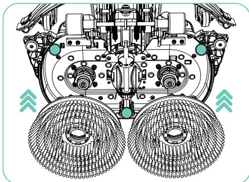
Remove the main tank and battery, gently lay the machine on its front. Push fit the brushes, clicking into place onto the motor chucks. To remove the brushes, place your fingers behind the brush deck in locations shown
