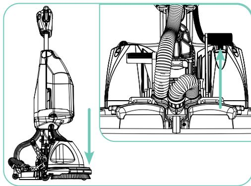
Lower the floor tool by pressing down on the left foot lever, lower the machine deck by pushing the right pedal forward.
