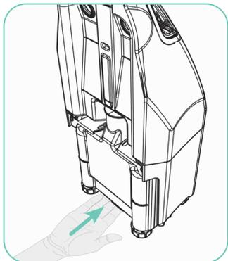
Tilt the tank assembly slightly forward and slide your hand under the tank.
