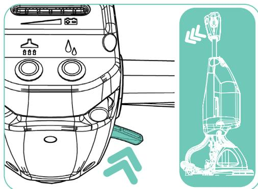
Standing behind the machine, pull the lever on the right hand side to lower the handle height.
