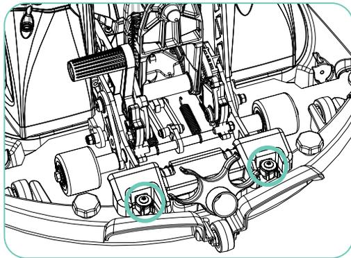
Push the floor tool carrier handle down, then mount the floor tool onto the retaining clips.
