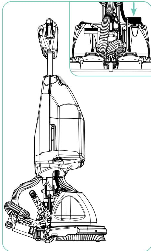
Press down on the foot pedal to raise the storage wheels.
