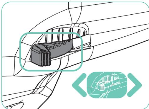
The dials on each side of the machine can be adjusted to set the water flow from the machine. Make sure they are both set the same
